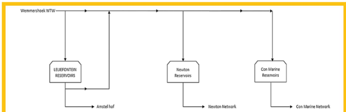
**FIGURE 1:** Existing Network Under Gravity Flow
