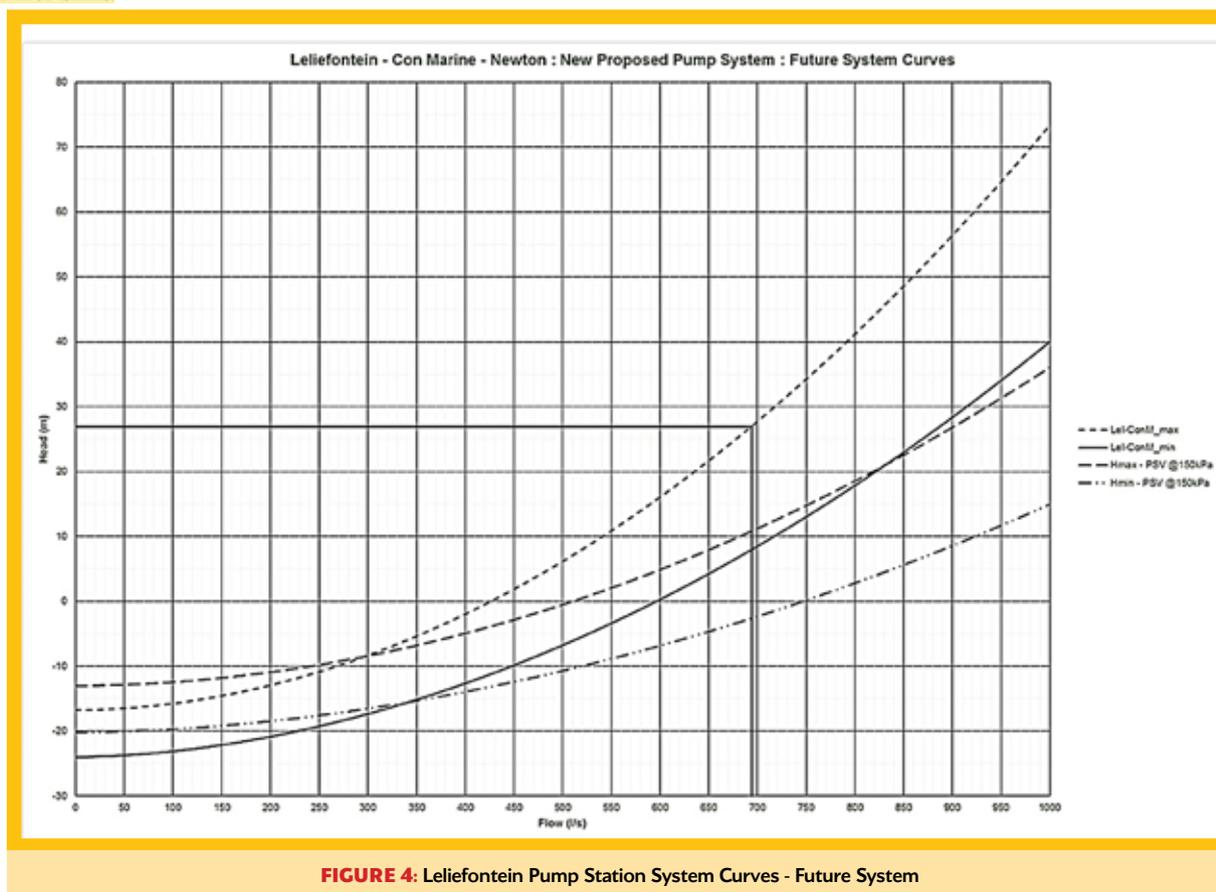
**FIGURE 4:** Leliefontein Pump Station System Curves - Future System
