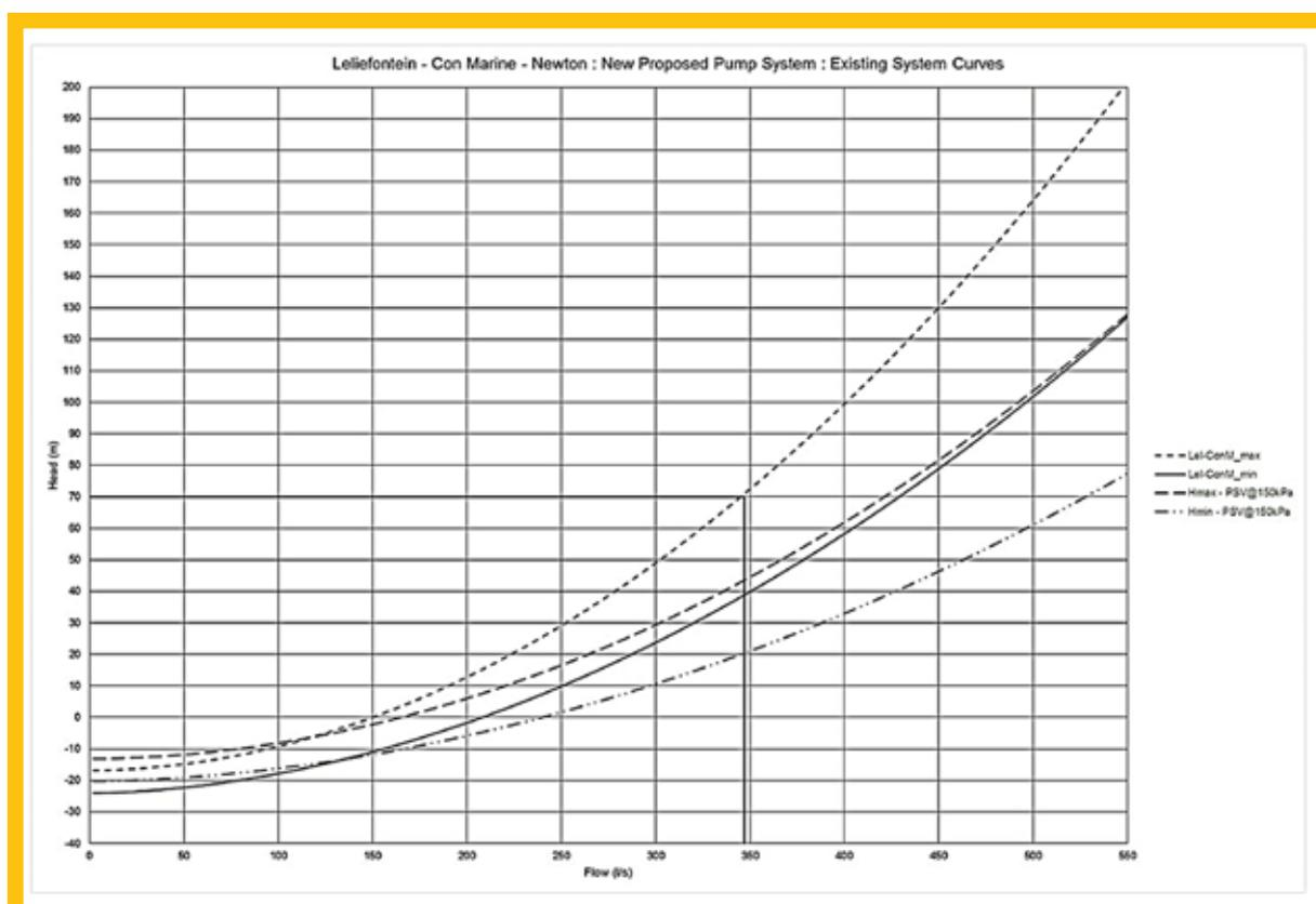
**FIGURE 3:** Leliefontein Pump Station System Curves - Initial System
