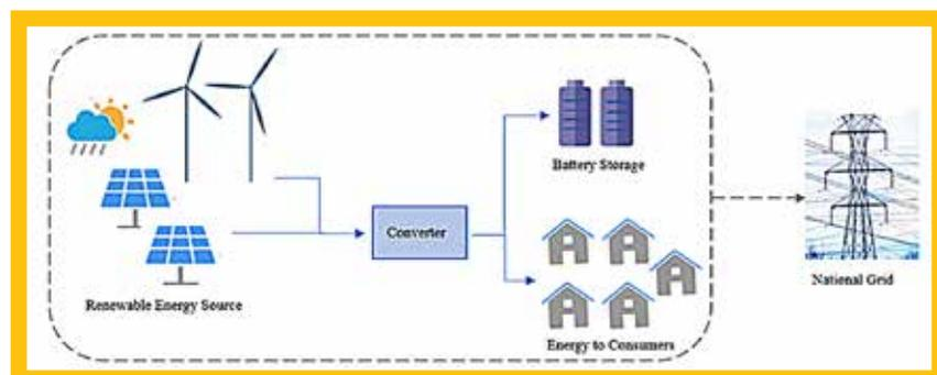
FIGURE 1: Typical Micro-grid from Renewable Energy Sources
