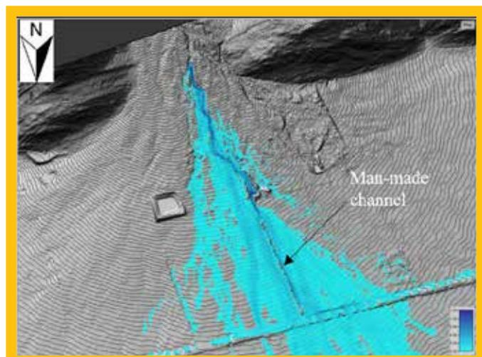
**FIGURE 2:** Simulated study area flow depths (m) at peak of the 20-year flood (50 m<sup>3</sup>/s)
