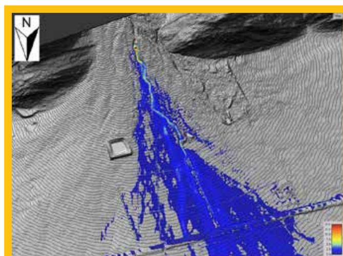
**FIGURE 5:** Simulated attenuation dam flow depths (m) at 20-year inflow peak (50 m<sup>3</sup>/s) and 2-year peak outflow (25 m<sup>3</sup>/s)
