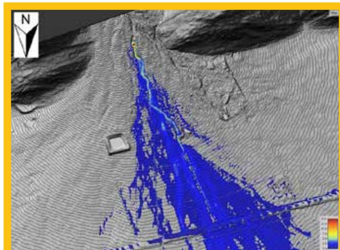
**FIGURE 3:** Simulated study area flow velocities (m/s) at peak of the 20-year flood (50 m<sup>3</sup>/s)
