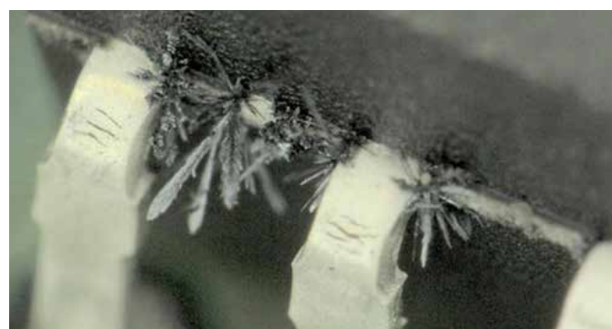
FIGURE 4: Cross section of a corroded copper track after mixed gas test (H 2 S (2.11 ppm) + SO 2 (10 ppm) + Cl 2 (0.1 ppm), 21 days) showing the build-up of corrosion
