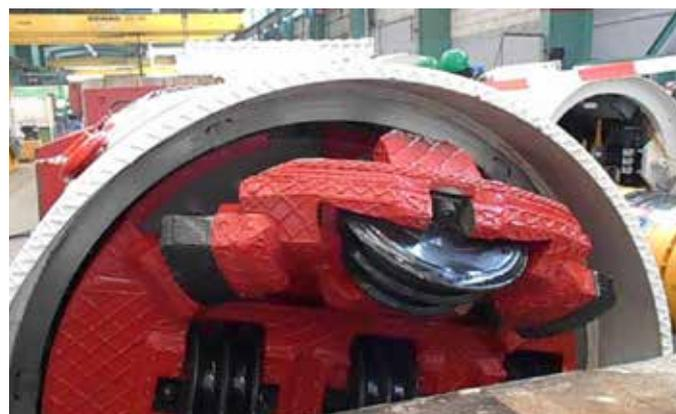
**FIGURE 13:** Foldable cutterhead of retractable AVN800
