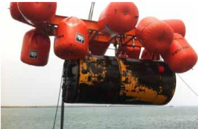
**FIGURE 11:** Recovery of tunnelling machine via airbags, lifting by crane in harbor
