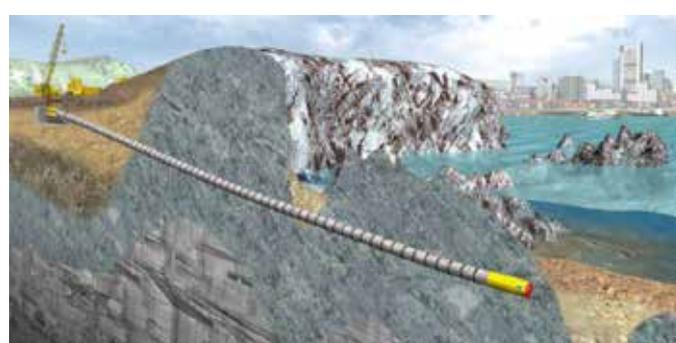
**FIGURE 8:** Function principle of Pipe Jacking marine outfall technology
