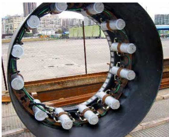
**FIGURE 5:** Interjacking station installed in pipe
