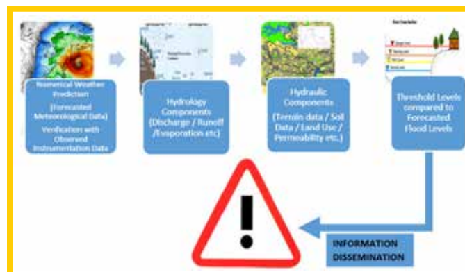
FIGURE 1: Basic Integration of Meteorological and Hydrological/ Hydraulic Components of Flood Early Warning Systems
