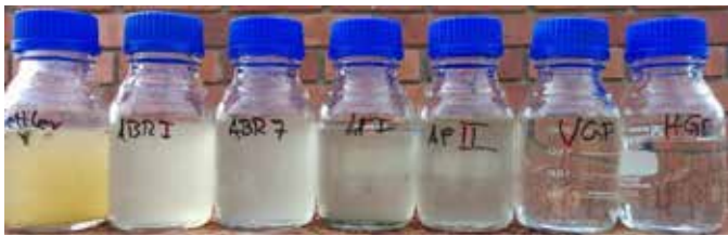
Figure 6: Samples collected from different modules of the Newlands Mashu DEWATS. Image: Bjoern Pietruschka.
