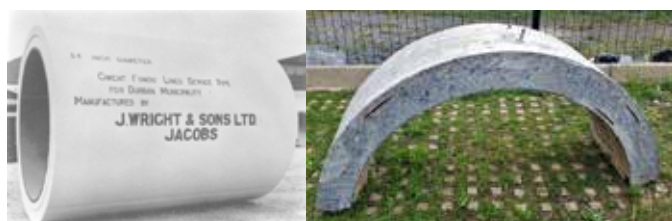
Figure 6: Precast concrete pipes with an internal lining of Ciment Fondu® mortar installed at Durban Municipality around 1955: left, at time of manufacturing in 1955; right, segment extracted in April 2018 in Point Road area with the Ciment Fondu® mortar lining still present.
