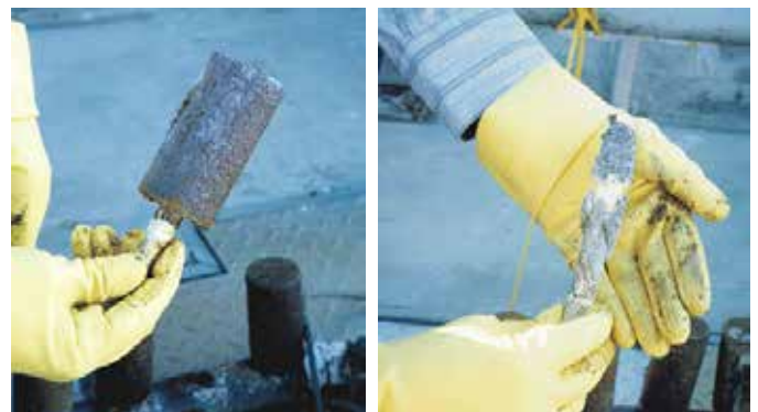
Figure 3: In situ specimens exposed for two years in the grit chamber of Monterey Wastewater Treatment Plant. Left: 100% CAC mortar. Right: OPC mortar
