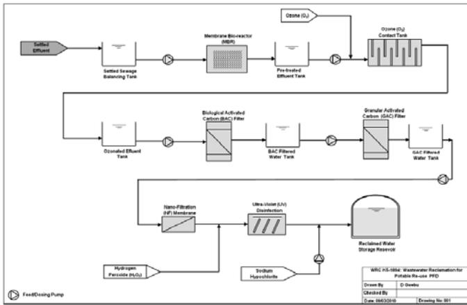
Figure 2: Water reuse process flow diagram (Acknowledgement: Umgeni Water)
