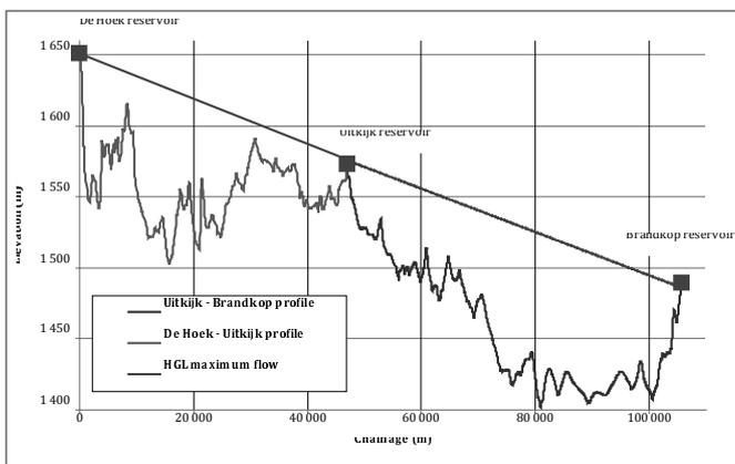
Figure 2: Longitudinal profile of the Caledon-Bloemfontein Pipeline
