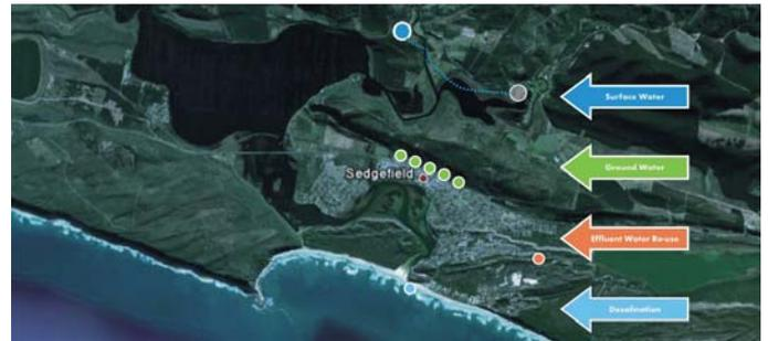
Figure 9: Sedgfield Water Augmentation Plan – Layout
