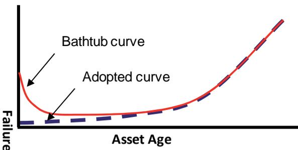
Figure 2: Bathtub curve and adopted probability of failure curve
