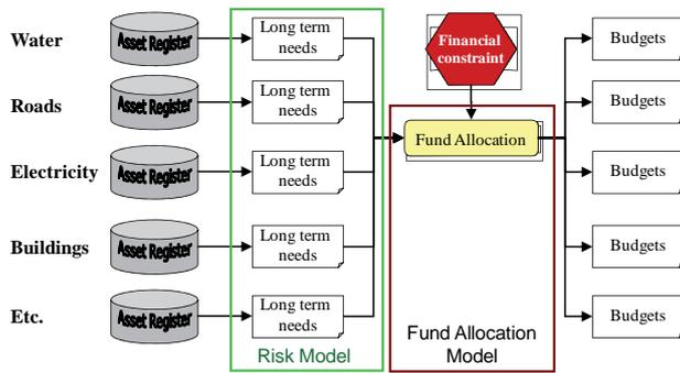
Figure 1: Conceptual design of the IMF
