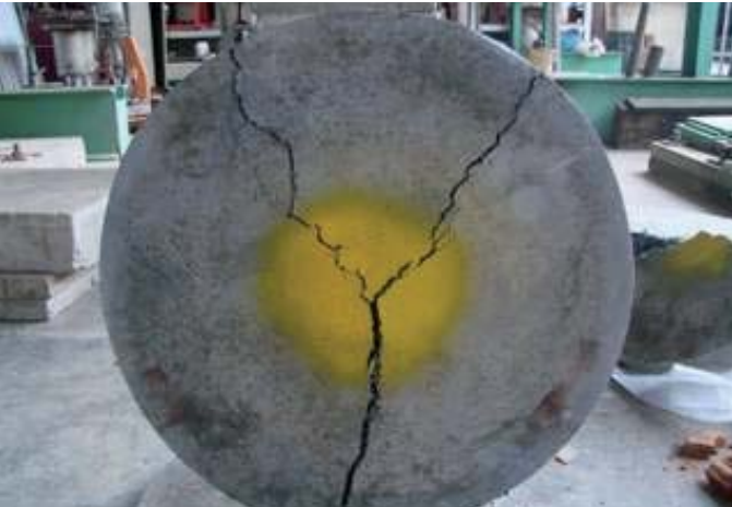
Figure 1: Testing of circular panels for energy absorption determination, modified ASTM C1550-05 test
