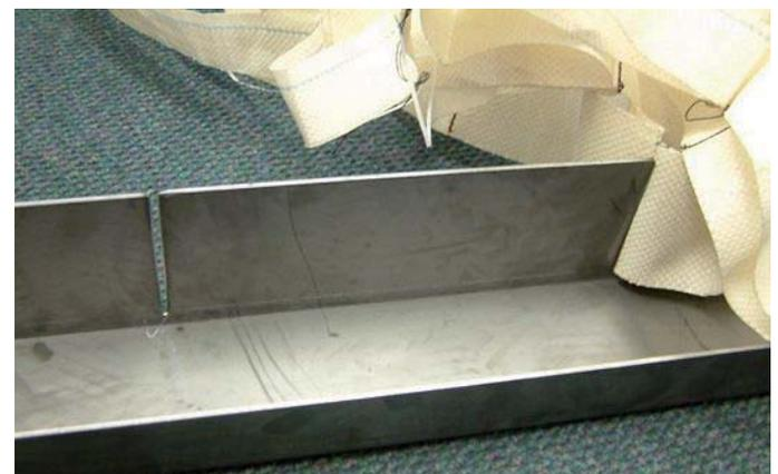
Figure 17: Geocells through side form slot
