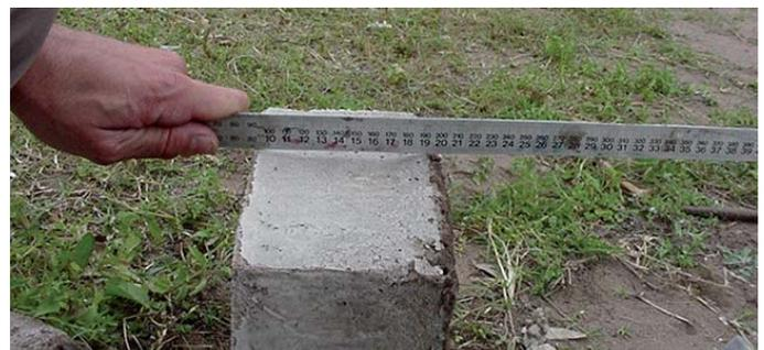
Figure 11: Interlock deformation of sidewalls
